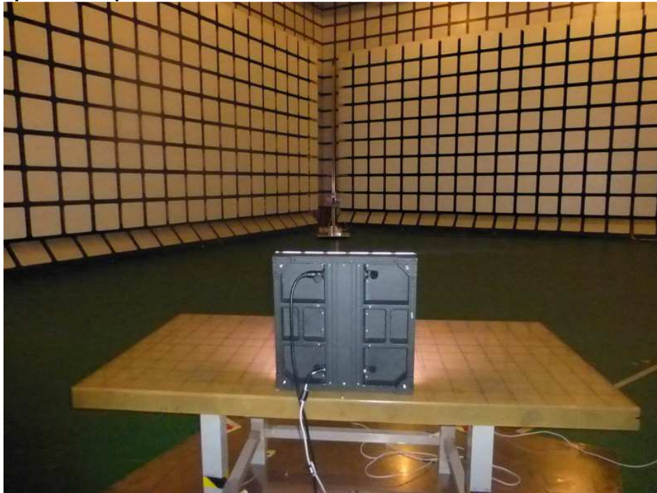
Photograph 3: Set-up for Radiated Emission
