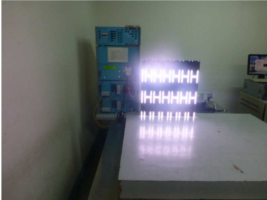
Photograph 1: Set-up for Harmonic and Voltage Fluctuations on AC Mains
