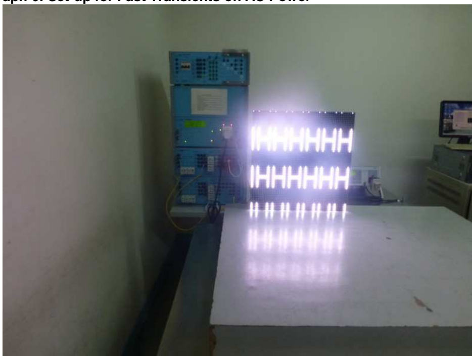
Photograph 6: Set-up for Fast Transients on AC Power
