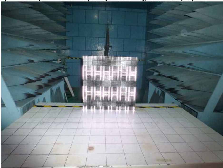
Photograph 4: Set-up for Radio-Frequency Electromagnetic Field (RS)
