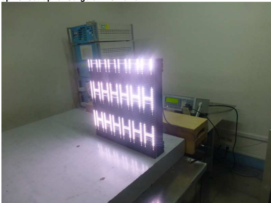
Photograph 8: Set-up for Surge on AC Power
